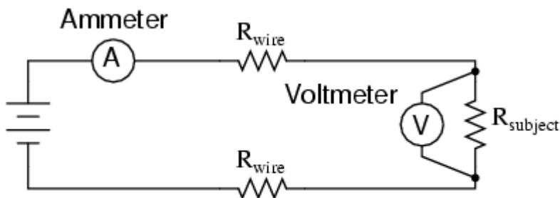
$$R_{subject} = \frac{\text{Voltmeter indication}}{\text{Ammeter indication}}$$
